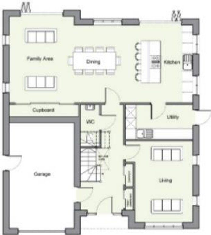
PROPOSED GROUND FLOOR PLAN - GIA 93m 2
